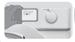
If you do not know the position of your NFC antenna, slightly move the smartphone in a circular motion over the SMART Fi+ logo until the App confirms the connection. In order for the data transfer to be successful, it is essential TO KEEP THE SMARTPHONE ON THE DASHBOARD DURING THESE THE FEW SECONDS OF THE PROCEDURE; a message on the device will inform about the correct outcome of the operation and advise you when it is possible to move the smartphone away.
