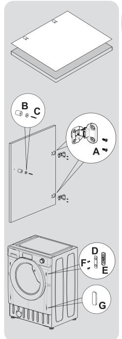
Mount the furniture door to the front of the washer using the hinges. Place the spacers under the hinges (I) and then fix in position with screw (H).
